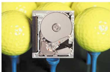
Fig. 9. (a) A photo of the Travelstar™ disc, manufactured by IBM. The disc spins as if it were on a record player and the information on it is read by a tiny GMR read head placed at the end of the “needle” of the record player. GMR read heads, like the one shown in the previous figure, can be manufactured on length scales on the order of 10 nm. The small size and high sensitivity of these devices have led to increased performance of magnetic information storage media. The disc shown above has an information storage density of 4.1 billion bits per square inch. (b) A marble model of a 1D magnetic nanowire array. By miscutting substrate surfaces to form atomic staircases, it is possible to grow parallel arrays of these nanowires using the stepped surface as a template [16].
